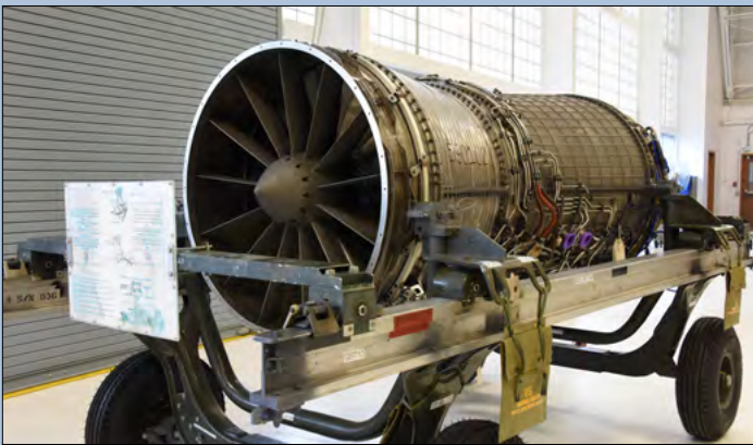
The F118-GE-101A non-afterburning engine is responsible for powering the U-2 Dragon Lady ultra-high altitude reconnaissance aircraft. (Air National Guard photo by Master Sgt. Patrick S. Kerr)
